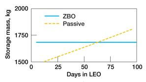
Figure 5.—Passive and ZBO cryogenic thermal storage mass versus duration for LH<sub>2</sub> storage in 3.3-m-diam tank.
