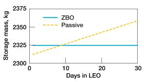
Figure 4.—Passive and ZBO cryogenic thermal storage mass versus duration for LCH<sub>4</sub> storage in 2.2-m-diam tank.
