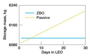
Figure 3.—Passive and ZBO cryogenic thermal storage mass versus duration for LO2 storage in 2.2-m-diam tank.
