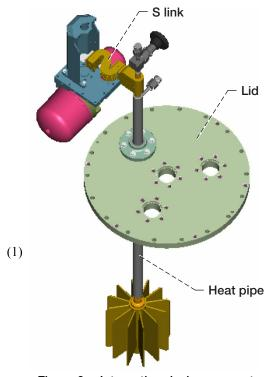
Figure 2.—Integration design connects cryocooler to propellant tank lid.
