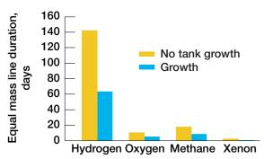
Figure 8.—Equal mass variation if tank growth to accommodate boil-off is not considered. If not, passive thermal control mistakenly appears to reduce mass to much longer storage duration than it should.
