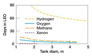
Figure 6.—Graphical composite that shows duration at which ZBO and passive storage mass is equal for a given tank size. Durations longer than these are predicted to save mass if ZBO is incorporated.
