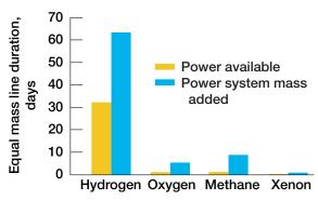
Figure 7.—Equal mass variation if power system is available and mass not included. If so, ZBO applicable for much shorter durations.
