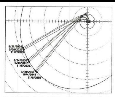
Fig. 7 Ecliptic projection of Makemake trajectory opportunities illustrating launch window periods for time of flight 16.16 years.
