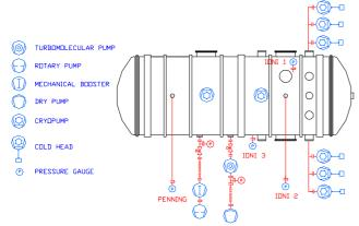
Figure 10 AEROSPAZIO's LVTF-1 test facility pumps arrangement [31]
