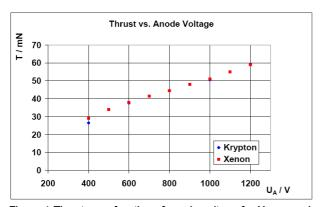
Figure 4 Thrust as a function of anode voltage for Xenon and Krypton operation at a mass flow of 1.89 and 1.81 mg/s, respectively.
