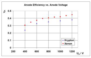
Figure 7 Anode efficiency as a function of anode voltage for Xenon and Krypton operation at a mass flow of 1.89 and 1.81 mg/s, respectively.
