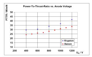
Figure 5 Power-to-thrust-ratio as a function of anode voltage for Xenon and Krypton operation at a mass flow of 1.89 and 1.81 mg/s, respectively.
