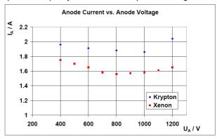
Figure 3 Anode current as a function of anode voltage for Xenon and Krypton operation at a mass flow of 1.89 and 1.81 mg/s, respectively.
