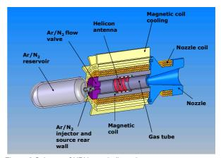
Figure 8 Scheme of HPH.com helicon thruster
