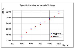
Figure 6 Specific impulse as a function of anode voltage for Xenon and Krypton operation at a mass flow of 1.89 and 1.81 mg/s respectively.
