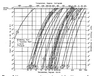
Figure 9 Vapor pressure -temperature relationship curves for common vacuum system gases [30]
