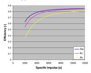
Figure 2 Representative ion thruster efficiency,  $\eta$ , for Xenon (Xe), Krypton (Kr), and Argon (Ar).
