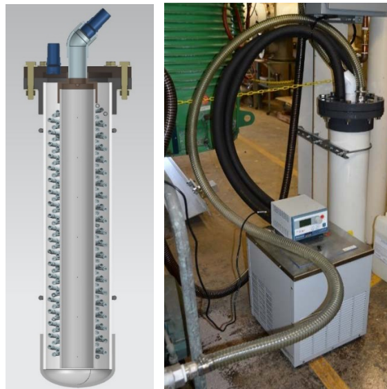
Figure 6: (Left) CAD model of the disposable iodine cold trap implemented for the durability demonstration. (Right) Photograph of the assembled cold trap chilled using a PolyScience 9712, installed between VF7 and a Stokes 149 vacuum pump.
