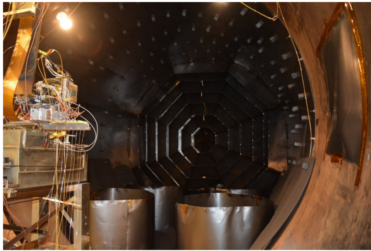
Figure 5: Iodine propulsion system assembly installed in GRC VF7 prior to 1,174-hour demonstration. All surfaces exposed to direct impingement of the iodine plume are protected with either grafoil, graphite felt, or solid graphite.
