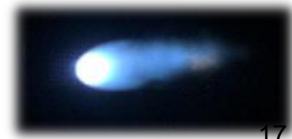
70° Sphere-Cone in Flight through CO 2 at 5 km/s
