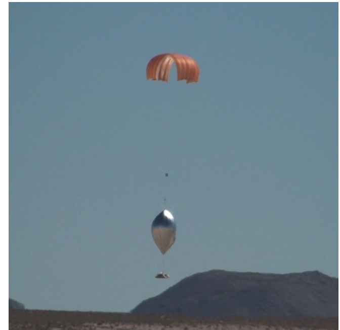
Second 5.5 m Venus prototype balloon during aerial deployment and inflation testing.
