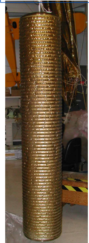
Prototype stainless steel bellows flotation device
