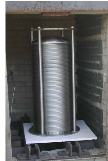
Prototype stainless steel bellows flotation device
